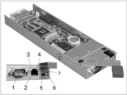
Figure 61: Management blade control and connection panel
